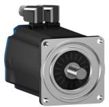
servo motor BSH, Lexium 05, 7.8N.m, 2500rpm, 100mm, keyed shaft, Sincos single turn, without brake, IP50
