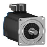
AC servo motor BSH, Lexium 05, 3.39N.m, 4000rpm, keyed shaft, without brake, IP50
