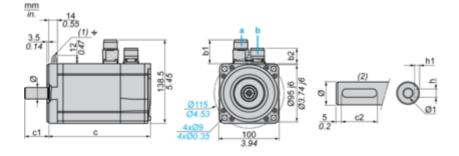
a: Power supply for servo motor brake
