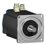
AC servo motor BSH, Lexium 05, 2.7N.m, 3000rpm, untapped shaft, with brake, IP50
