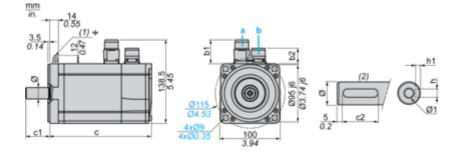
a: Power supply for servo motor brake
