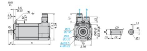
a: Power supply for servo motor brake
