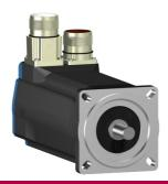
AC servo motor BSH, Lexium 05, 2.12N.m, 6000rpm, keyed shaft, with brake, IP50
