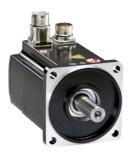
servo motor BMH, Lexium 32, 62.5Nm, 3800rpm, untapped shaft, with brake, IP65, IP67, 16bit encoder, straight
