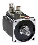
servo motor BMH, Lexium 32, 34.4Nm, 3800rpm, keyed shaft, without brake, IP65, IP67, 128 multiturn encoder
