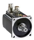
servo motor BMH, Lexium 32, 34.4Nm, 3800rpm, keyed shaft, without brake, IP65, IP67, 128bit encoder
