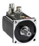
servo motor BMH, Lexium 32, 34.4Nm, 3800rpm, untapped shaft, without brake, IP65, IP67, 128 multiturn encoder
