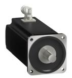
servo motor BMH, Lexium 32, 100Nm, 3000rpm, keyed shaft, with brake, IP65, IP67, 128bit encoder
