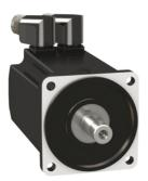
servo motor BMH, Lexium 32, 6Nm, 6000rpm, keyed shaft, without brake, IP65, IP67, 16 multiturn encoder
