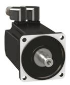
servo motor BMH, Lexium 32, 6.2Nm, 6000rpm, keyed shaft, without brake, IP54, 128bit encoder
