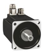
servo motor BMH, Lexium 32, 3.4Nm, 6000rpm, keyed shaft, without brake, IP54, 128 multiturn encoder, straight
