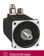
servo motor BMH, Lexium 32, 3.4Nm, 6000rpm, untapped shaft, with brake, IP54, 16bit encoder, straight
