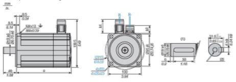
a: Power supply for servo motor brake
