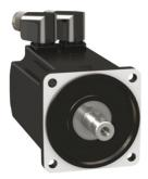
servo motor BMH, Lexium 32, 3.3Nm, 6000rpm, keyed shaft, without brake, IP65, IP67, 128 multiturn encoder
