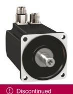
servo motor BMH, Lexium 32, 3.3Nm, 6000rpm, untapped shaft, with brake, IP65, IP67, 16 multiturn encoder, straight
