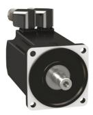
servo motor BMH, Lexium 32, 3.3Nm, 6000rpm, untapped shaft, with brake, IP65, IP67, 16bit encoder
