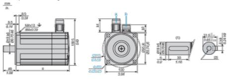
a: Power supply for servo motor brake
