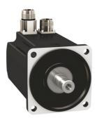
servo motor BMH, Lexium 32, 3.3Nm, 6000rpm, keyed shaft, without brake, IP54, 128bit encoder, straight
