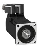
servo motor BMH, Lexium 32, 3.4Nm, 8000rpm, untapped shaft, with brake, IP65, IP67, 16bit encoder
