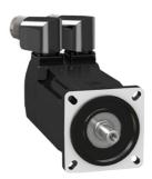
servo motor BMH, Lexium 32, 3.4Nm, 8000rpm, keyed shaft, with brake, IP54, 16 multiturn encoder
