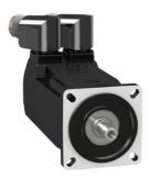
servo motor BMH, Lexium 32, 3.4Nm, 8000rpm, keyed shaft, with brake, IP54, 16bit encoder
