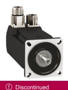
servo motor BMH, Lexium 32, 3.4Nm, 8000rpm, untapped shaft, with brake, IP54, 128 multiturn encoder, straight, 3 phases
