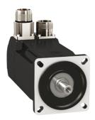
servo motor BMH, Lexium 32, 2.5Nm, 8000rpm, untapped shaft, without brake, IP65, IP67, 16bit encoder, straight
