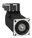
servo motor BMH, Lexium 32, 2.5Nm, 8000rpm, keyed shaft, with brake, IP65, IP67, 16bit encoder, 3 phases
