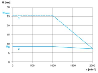
Servo Motor with LXM28AU10 ••• Servo Drive
