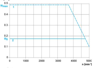
Servo Motor without shaft sealing ring and LXM28AU01  $\bullet \bullet \bullet$  Servo Drive M [Nm]
