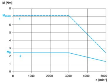
Servo Motor with LXM28AU04 ••• Servo Drive
