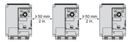
Only Possible at Ambient Temperature Less or Equal to 50 °C (122 °F)
