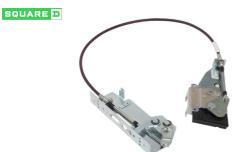
Disconnect mechanism, cable operated, cable operator, 48 inch cable, for 9422TCF, TCN, TDF, TDN, TEF or TEN switch
