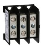
Power distribution block, Linergy, 3 pole, 1 line, 1 load, 115A CU, 90A AL, 600 V
