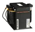
Transformer, Type T, industrial control, 2000VA, 1 phase, 550/575/600V primary, 120/240V secondary, 115C rise
