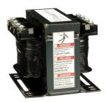
Transformer, Type T, industrial control, 150VA, 1 phase, 240x480V primary, 24V secondary, 55C rise
