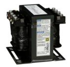
Transformer, Type T, industrial control, 150VA, 1 phase, 120V primary, 12/24V secondary, 55C rise
