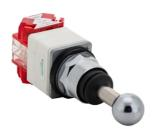
Joystick controller, Harmony 9001K, metal, 30mm, 4 directions, spring return to center, 2 CO
