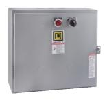
Contactor, Type L, multipole lighting, electrically held, 30A, 10 pole, 600 V, 277 VAC 60 Hz coil, NEMA 1, +option
