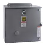
Contactor, Type L, multipole lighting, electrically held, 30A, 10 pole, 600 V, 110/120 VAC 50/60 Hz coil, NEMA 3R/12
