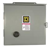
NEMA Starter, Type S, reversing, horizontal, Size 1, 27A, 10 HP at 575 VAC, 5 kA SSCR, 3 phase, 3 pole, melting alloy overload, 600 VAC coil, NEMA 12
