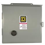
NEMA Starter, Type S, reversing, horizontal, Size 1, 27A, 10 HP at 575 VAC, 5 kA SSCR, 3 phase, 3 pole, melting alloy overload, 120 VAC coil, NEMA 12
