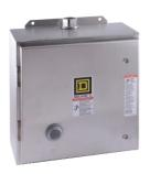
NEMA Starter, Type S, reversing, horizontal, Size 0, 18A, 5 HP at 575 VAC, 5 kA SSCR, 3 phase, 3 pole, melting alloy overload, 208 V coil, NEMA 4/4X
