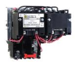
NEMA Starter, Type S, reversing, horizontal, Size 0, 18A, 5 HP at 575 VAC, 5 kA SSCR, 3 phase, 3 pole, melting alloy overload, 208 VAC coil, open
