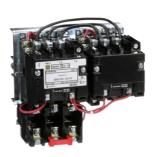
NEMA starter, Type S, reversing, horizontal, Size 0, 18A, 5HP at 575VAC, 5kA SSCR, 3 phase, 3 pole, melting alloy overload, 120VAC coil, open
