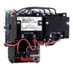
NEMA Starter, Type S, reversing, horizontal, Size 0, 18A, 5 HP at 575 VAC, up to 100 kA SCCR, 3 phase, 3 pole, Motor Logic SSOLR, 120 VAC coil, open
