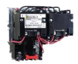
NEMA Starter, Type S, reversing, horizontal, Size 0, 18A, 2 HP at 230 VAC, 5 kA SSCR, 1 phase, 3 pole, melting alloy overload, 120 VAC coil, open
