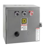
NEMA Starter, Type S, reversing, horizontal, Size 0, 18A, 5 HP at 575 VAC, up to 100 kA SCCR, 3 phase, 3 pole, Motor Logic SSOLR, 208 VAC coil, NEMA 1
