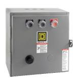
NEMA Starter, Type S, reversing, horizontal, Size 0, 18A, 5 HP at 575 VAC, 5 kA SSCR, 3 phase, 3 pole, melting alloy overload, 480 VAC coil, NEMA 1
