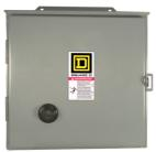
NEMA Starter, Type S, reversing, horizontal, Size 0, 18A, 5 HP at 575 VAC, up to 100 kA SCCR, 3 phase, 3 pole, Motor Logic SSOLR, 480 V coil, NEMA 12
